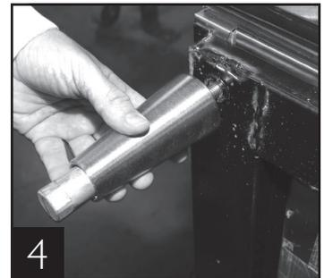
4 Thread leg into cabinet bottom frame rail.
