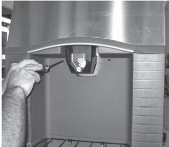
3. With the screws out remove the front panel by grasping both sides and pulling towards you until it is clear of the ice chute, then pull the panel up and out.
