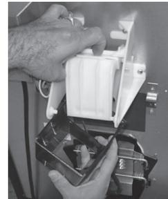
6. Put the new ice chute into place by lifting the door lock and door lock assembly. Rotate the chute counter clockwise in an up and away from you motion and snap the bracket pins into place. Replace the metal bracket clip.
