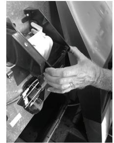
7. As you lift the front panel up onto the lower brackets, slide the chute through the opening in the front panel. Rest the panel on the lower brackets.
