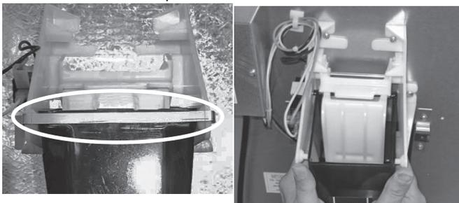
5. Lift the door lock and rotate the ice chute clockwise while pulling towards you in a slightly downward motion to complete removal.
