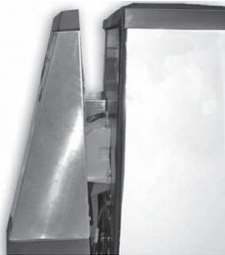
4. Remove the metal outer bracket clip, then use your thumbs to spread the bracket and unhinge the ice chute from the bracket pins.
