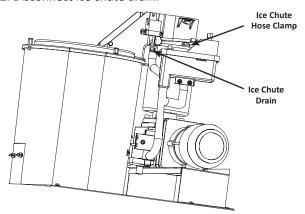
13. Lift up on ice chute to remove. The ice chute must be removed before the bin cover can be removed.
