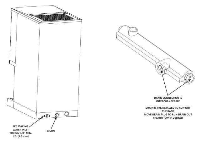
**Typical Water Supply Drain Installation**
