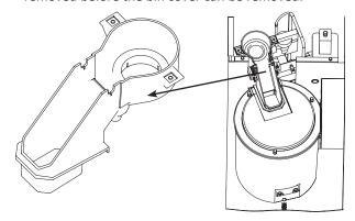
14. The ice chute can be cleaned in place. If complete removal is desired, use a Phillips screwdriver to remove the Hall Effect switch assembly from the ice chute.
