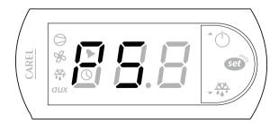
This means the <u>Temperature Set button</u> **Set** was held down longer than 3 seconds. To exit this mode and restart, press <u>Temperature Set Button</u> **Set**
